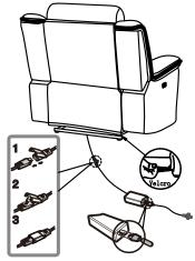
Safety Note: Transformer and cables are not to be placed under or within the recliner structure.
